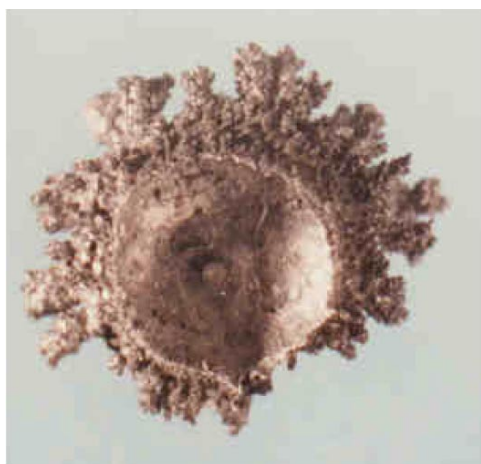
Figure 5. The result of GaN synthesis from the liquid Ga and N 2 plasma. The liquid has been pushed out from the initial droplet covered by GaN crust, by the growing N 2 bubbles.
